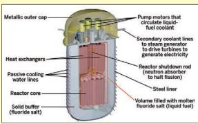
Generic design of a molten salt reactor
