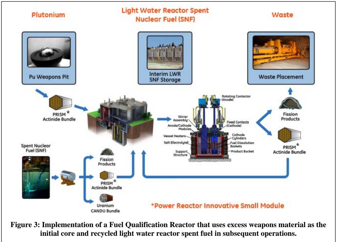
**Figure 3: Implementation of a Fuel Qualification Reactor that uses excess weapons material as the initial core and recycled light water reactor spent fuel in subsequent operations.**
