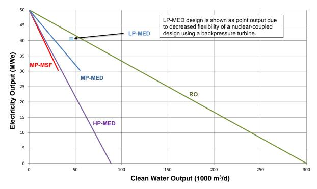
Fig. 5 Relationship between electricity and water output from a single NuScale module coupled to a variety of membrane and thermal distillation desalination processes.
