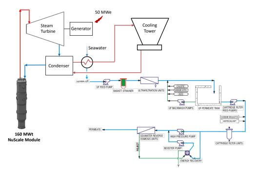
Fig. 4 NuScale plant coupled to an RO desalination cycle.
