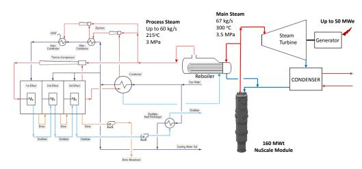
Fig. 2 Process diagram for a NuScale module coupled to an MED-TC distillation cycle.
