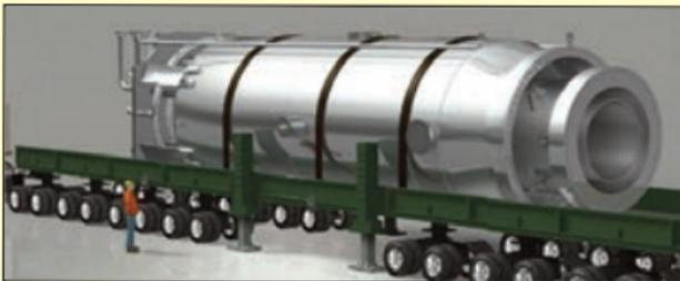
Concept drawing of a NuScale SMR power module transportable via specialized trailer or rail transport.
