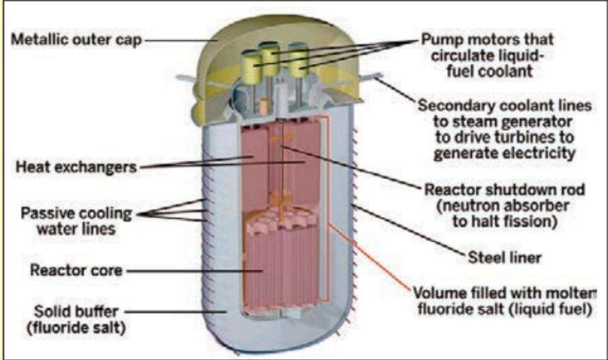
Generic design of a molten salt reactor
